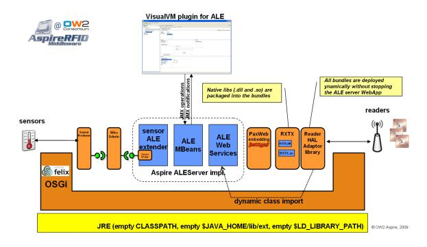
Figure : architecture of the ALEServer' OSGi profile (HiRes picture)
