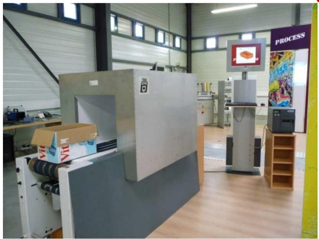
Reception check on a box with a tunnel reader
